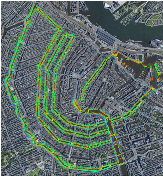
Fig. 8: Map of LIO-SAM aligned with Google Earth.
